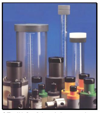
Griffco high flow diaphragm back pressure valves are designed to enhance the performance of higher flow, continuos feed pumps that require a constant head pressure, while also acting as an anti-syphon valve. Larger orifice sizes make the valve ideal for use with higher viscosity fluids. Wetted materials include: PVC, CPVC, PP, PVDF, PTFE, 316 SS, A 20 and Hast. C. Available in ½", ¾" and 1" sizes.
