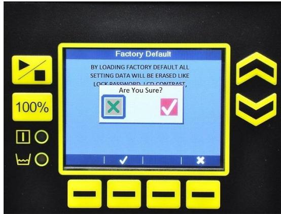
Figure 16: Factory Default Reset Verification
