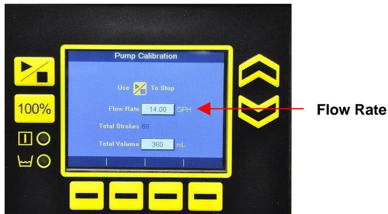
**Figure 25:** Pump Calibration (Set Flow Rate)
