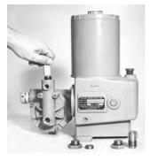
FIGURE VI VALVE CARTRIDGE REMOVAL, METAL HEAD PUMP
