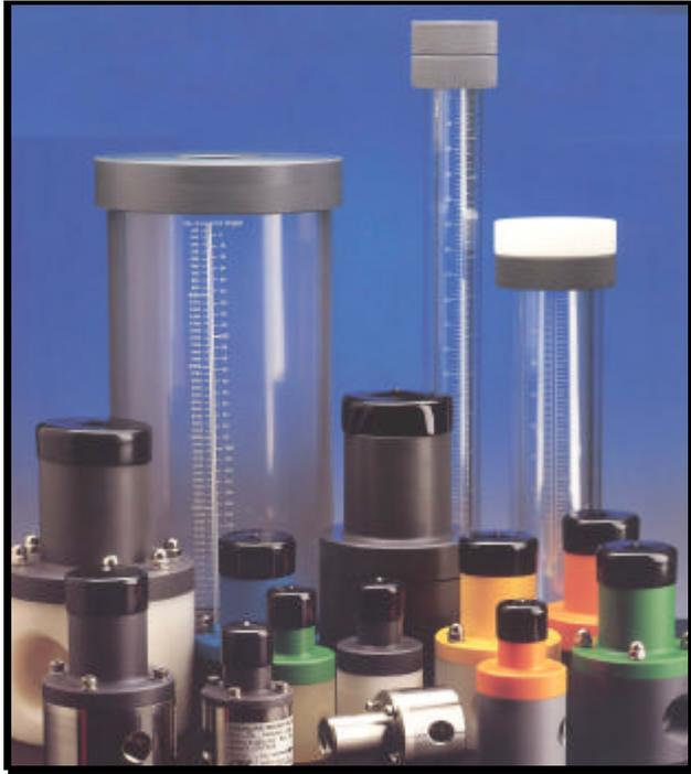
Griffco high flow diaphragm back pressure valves are designed to enhance the performance of higher flow, continuous feed pumps that require a constant head pressure, while also acting as an anti-syphon valve. Larger orifice sizes make the valve ideal for use with higher viscosity fluids. Wetted materials include: **PVC, CPVC, PP, PVDF, PTFE, 316 SS, A 20 and Hast. C.** Available in 1/2", 3/4" and 1" sizes.
