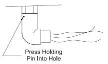
6. The elbow is now secured to the pump.
