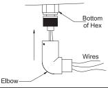
5. While holding the elbow securely, press the holding pin into the hole and tap into place using a small hammer.
