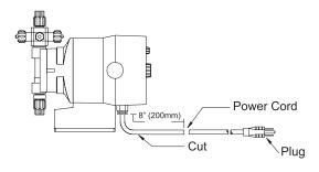
2. Strip away the outer cord jacket, leaving 1/2" (13 mm) intact below the strain relief.
