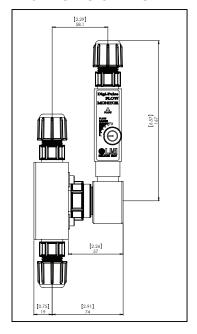
Right Angle Adapter with 4-Function Valve FIG 2
