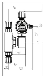
Right Angle Adapter with DIGI-PULSE™ and 4-Function Valve FIG 3
