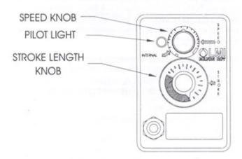
For maximum volumetric efficiency leave Stroke Length Knob at its maximum setting (100) unless it is impossible to reduce the pump's output sufficiently by turning Speed Knob. If Stroke Length Knob must be adjusted in order to reduce pump output, avoid turning it below minimum setting indicated on dial: doing so reduces the length of the stroke causing volumetric efficiency loss.
