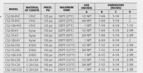
tSpecial lengths are available up to 24" for CPVC & Kynar; up to 36" for 3165S & Carpenter 20-Cb3.
