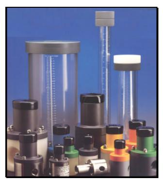
Griffco diaphragm back pressure valves are designed to enhance the performance of chemical feed systems by applying a continuous back pressure to the chemical feed pump, while also acting as an anti-syphon valve. Robust construction ensures reliability in the rigorous service of municipal and industrial applications. Wetted materials include: PVC, CPVC, PP, PVDF, PTFE, 316 SS, A 20 and Hast. C. Available sizes: 1/2 - 2".
