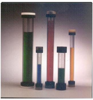
Griffco Borosilicate Glass Calibration Cylinders are designed to enhance the performance of chemical feed systems by providing a verification of the flow rate of the chemical feed pump. Constructed of borosilicate glass and a choice of 5 end cap materials, (PVC, PTFE, PVDF, 316 SS, A20) these cylinders are suitable for use with most chemicals. 6 sizes; 100 mL, 200 mL, 500 mL, 1000 mL, 2000 mL, 4000 mL.
