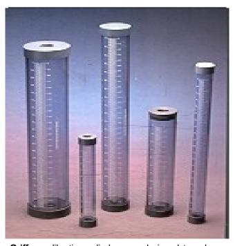
**Griffco** calibration cylinders are designed to enhance the performance of chemical feed systems by providing a verification of the flow rate of the chemical feed pump. Robust construction of clear PVC with an easy to read graduation in mls and gph. Available in three models: EZ-Clean, Vented, and Open Top; and 6 sizes; 100 mL, 200 mL, 500 mL, 1000 mL, 2000 mL, 4000 mL, 10,000 mL, and 20,000 mL.
