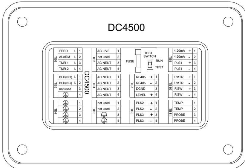
**Wiring diagram for external pulse output control.**
